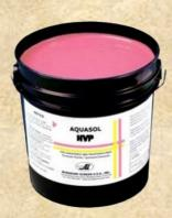
Murakami Aquasol HVP is a high viscosity emulsion to create extremely durable stencils for all ink systems. It has a more transparent quality that can help when registering by hand on press. Exposes fast and provides one of the most durable stencils possible for difficult inks like water base and discharge when combined with diazo additive and hardened with Murakami Hardeners.
